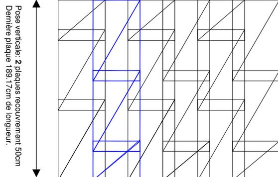
Pose verticale: 2 plaques recouvrement 50cm
