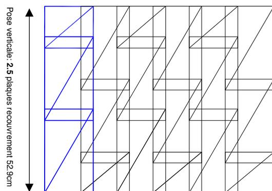
Pose verticale: 2.5 plaques recouvrement 52.9cm
